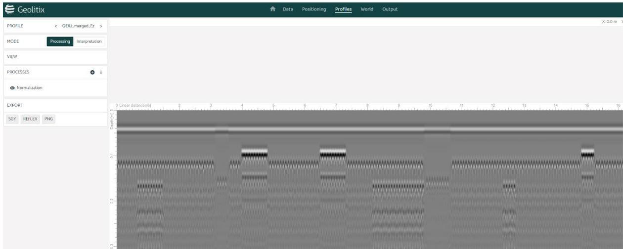
Figure 3: extract from the simulated data showing two voids, above and below the bars, and an area of 'wet' concrete.
