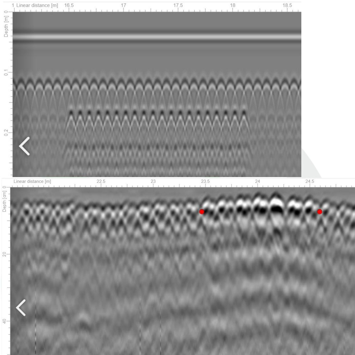
Figure 6: simulated data above and collected below, showing voids below the bars
