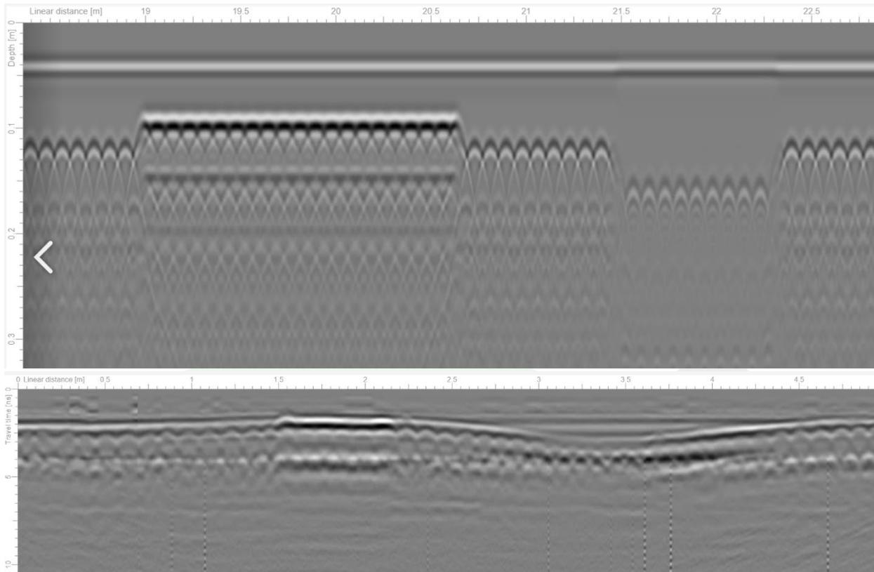
Figure 5: Simulated data above and real data below showing an air void above the bars with an area of 'wet' concrete.
