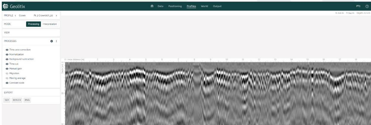
Figure 4: Collected site data with postprocessing showing several variations in the data, including voiding and variations in the dielectric of the concrete.
