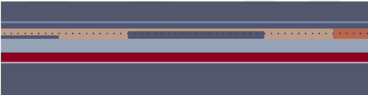
*Figure 2: Example model run through gprMax: 150mm of concrete (orange) with bars (blue dots) at 100mm centres. This sits on the original pipe (light blue) and some earth (red). To this we have added voids (the dark blue) and 'wet' patches (orange) (areas of higher conductivity and amplitude).*
